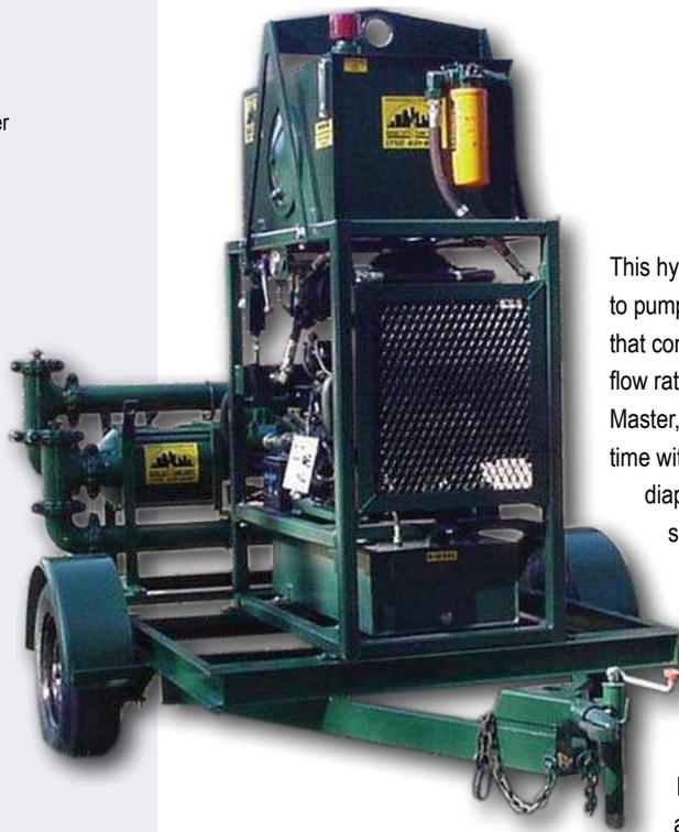
This hydraulically-driven, piston pumping system is designed to pump heavy sludges, slurries and other viscous materials that contain solids and impurities. The pumping system has a flow rate up to 250 gallons per minute. The self-priming Sludge Master, which is virtually leak proof, can dry run for a limited time without damage. It features low maintenance with no diaphragms that can burst under pressure or mechanical seals to fail.
